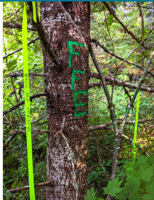
The flow feature extent (FFE), shown appropriately marked according to the survey protocols (permanent tree marking paint optional), is the upstream end of flowing water greater than 25 feet in length within a distinct stream bed and banks. In Phase 1, the only FFE point required is at the uppermost FFE, which is considered the end of perennality.
