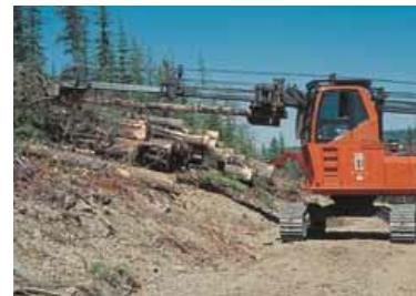
The stroke-boom delimber operates at the landing or roadside, removing tree limbs and top, cutting the stem into logs and stacking them.
