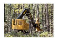
These evenly distribute the machine's weight to reduce soil compaction. Roads, trucks and other equipment are also kept away from streams.
