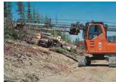
The stroke-boom delimer operates at the landing or roadside, removing tree limbs and top, cutting the stem into logs and stacking them.
