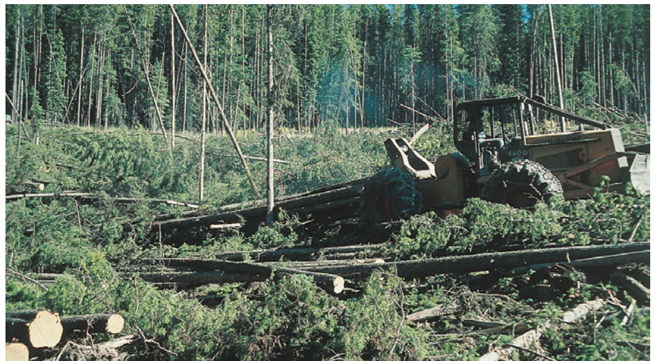
Skidders or dozers drag logs from the forest to the log landing. To reduce soil disturbance, rubber-tired skidders or crawler tractors should be kept on skid trails. Winch line and chokers pull logs to the machine.
